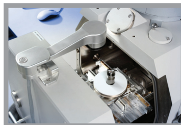
Nav-Cam. The fixed position of the Nav-Cam enables repeatable navigation without realignment.
