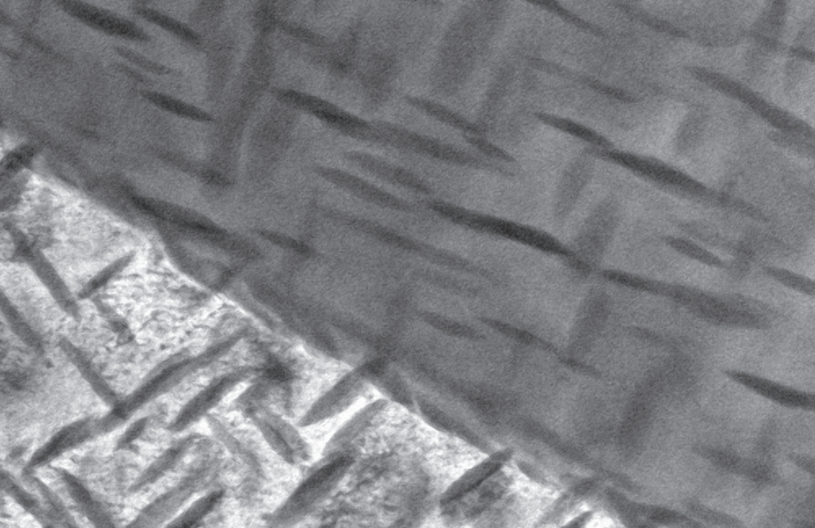
^ High-resolution bright field STEM image of a NiTiZr shape memory alloy. This material is a lightweight, solid-state alternative to conventional actuators such as hydraulic, pneumatic, and motor-based systems.
